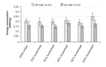
FIGURE 5. Effect of die outlet hole diameter on electrical energy consumption during extrusion of maize-buckwheat mixtures. of energy consumption occurred at 100% buckwheat content for die hole diameter of 12 mm (Figure 5).
