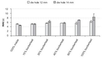
FIGURE 4. Effect of die outlet hole diameter on water absorption index (WAI) of maize-buckwheat extrudate.
