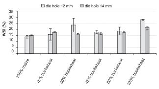
FIGURE 3. Effect of die outlet hole diameter on water solubility index (WSI) of maize-buckwheat extrudate.
