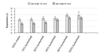
FIGURE 1. Effect of die outlet hole diameter on expansion ratio of maizebuckwheat extrudate.
