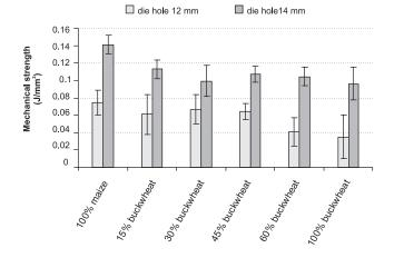
FIGURE 2. Effect of die outlet hole diameter on mechanical strength index of maize-buckwheat extrudate.
